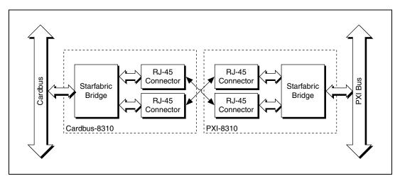
Figure 1-1. NI CardBus-8310-to-PXI Block Diagram
